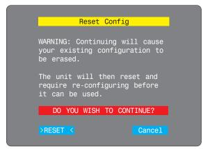
5 Remove power, return the mini switch 1 to its OFF position and then reapply power. The locally connected monitor should display the first screen of the initial configuration sequence.
